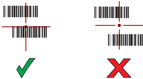
Figure 119: Pick List Mode with Multiple Bar Codes in Aiming Pattern
